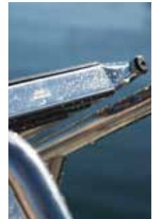
Pivoting handles For better stowing. (BUT45R)
