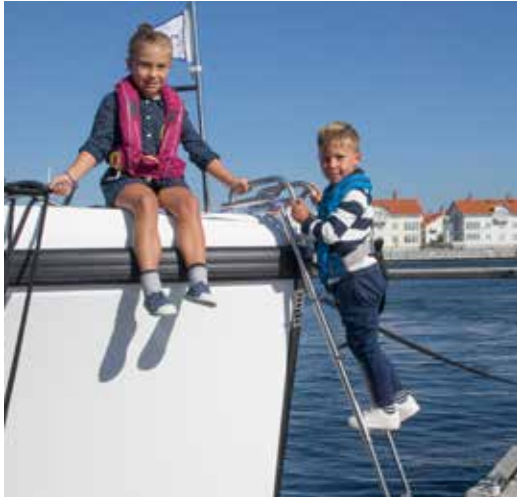
Ladders for bowsprits, with sturdy handles. Hook onto the bowsprit or on deck.
